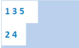
Artex Textured Finish (powder) should be applied liberally by brush or roller, covering about 1m x 0.5m at a time across the narrowest width of a room, then textured to the desired pattern. Whilst the material is still wet continue this way, blending in successive bands, until the entire surface has been textured. A 13mm brush margin should be made around all perimeter edges.
