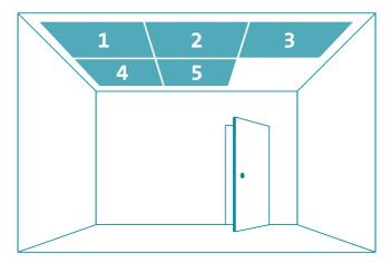
Apply a generous, even coat of the mix by brush or roller in a band about 1 x 0.5 metres across the ceiling width or down the wall (a single band can be applied from ceiling to skirting). Texture this area and draw a brush margin (13-25mm) using a small brush along the edges of the ceiling or wall to form a narrow border. Apply the next band and blend in with the previously textured area, again forming the margin line at the edges.
